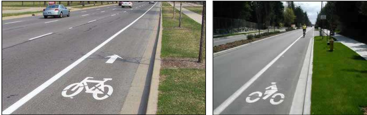
Figure 6.14: Examples of Bike Line Roadway Markings
